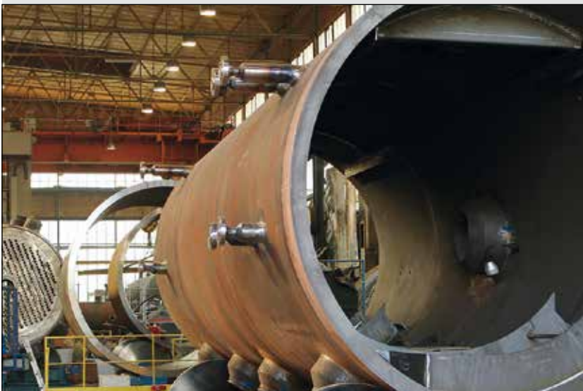
Manufacturing of steam drum
