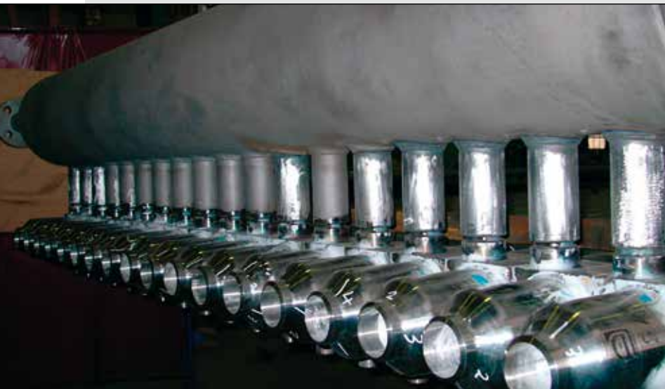
Gas inlet heads with BfW supply header
