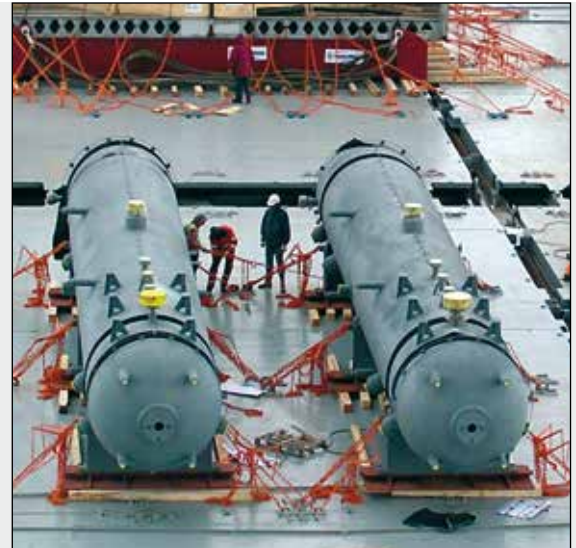
Shipped steam drums
