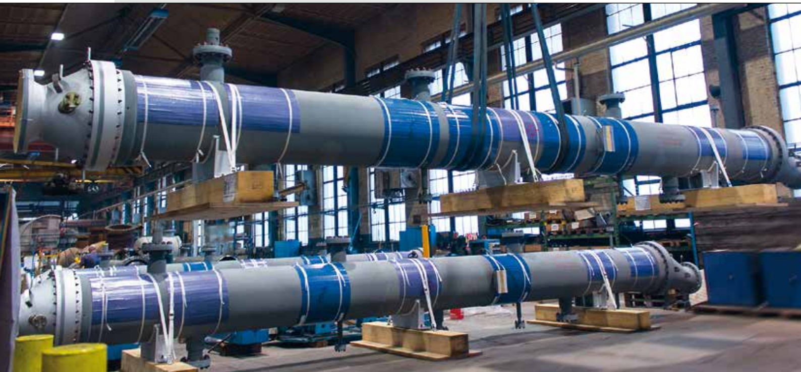
Manufacturing of "Tunnelflow" Transfer Line Exchangers
