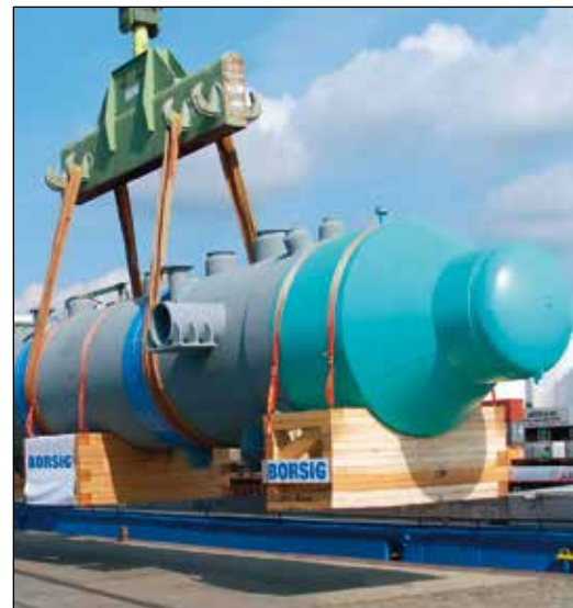
Process gas waste heat boiler
