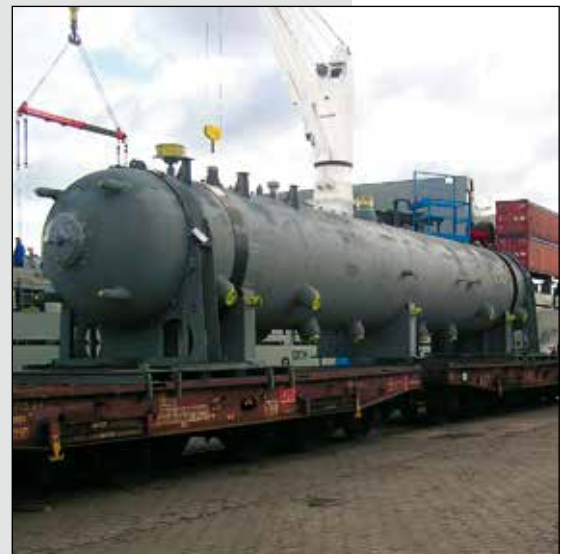
Steam drum ready for shipment
