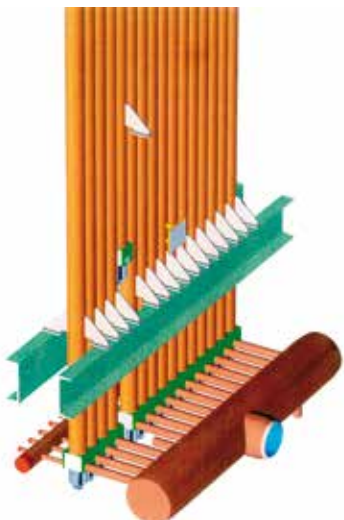
Cutting process / waterside connections lifting upwards
