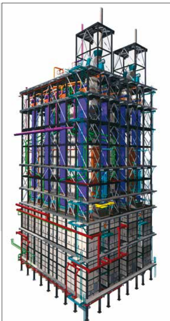
Computer simulation of two naphtha cracking furnaces
