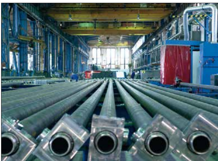
Double pipe elements in the workshop
