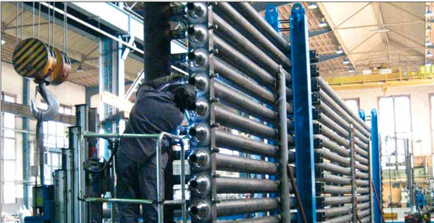
Manufacturing of "Linear" Transfer Line Exchangers
