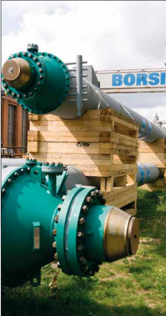
“Tunnelflow” TLEs ready for shipment
